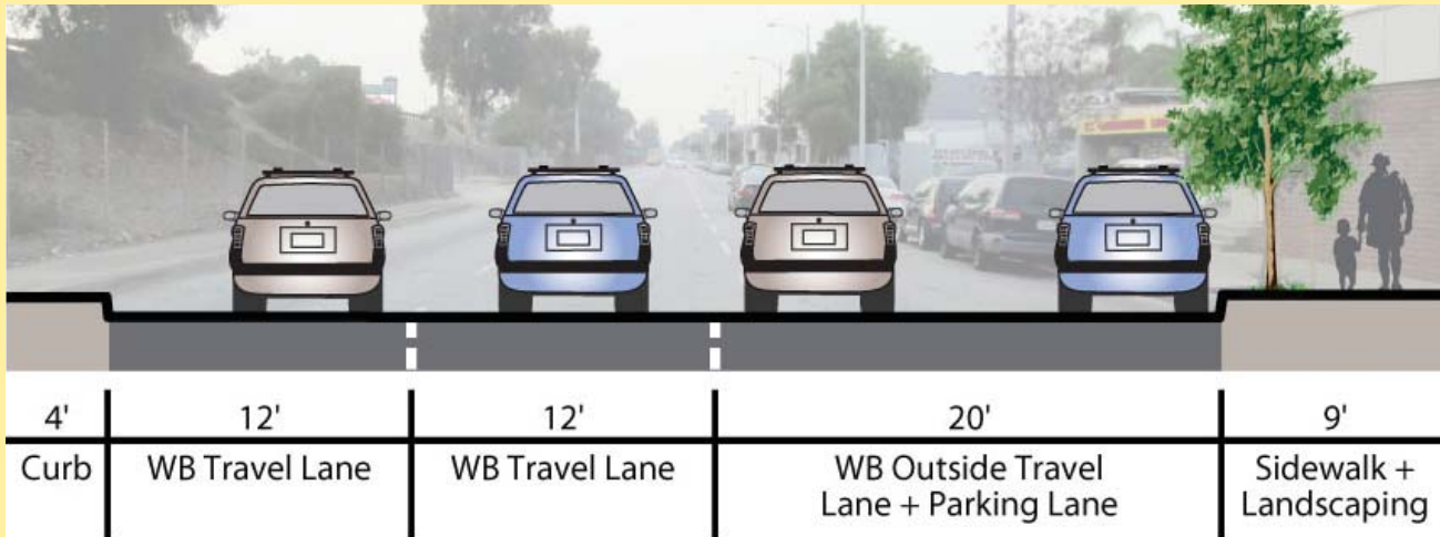
Existing Street Cross-Section
