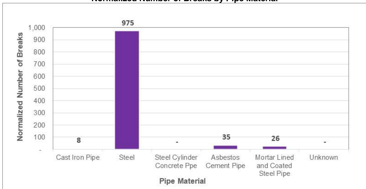
Figure 10-1 Normalized Number of Breaks by Pipe Material
